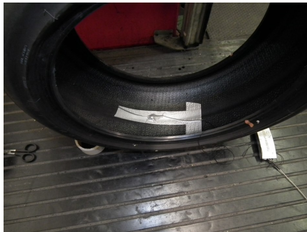
Figure 1. TCA's accelerometer installed on tyre liner
